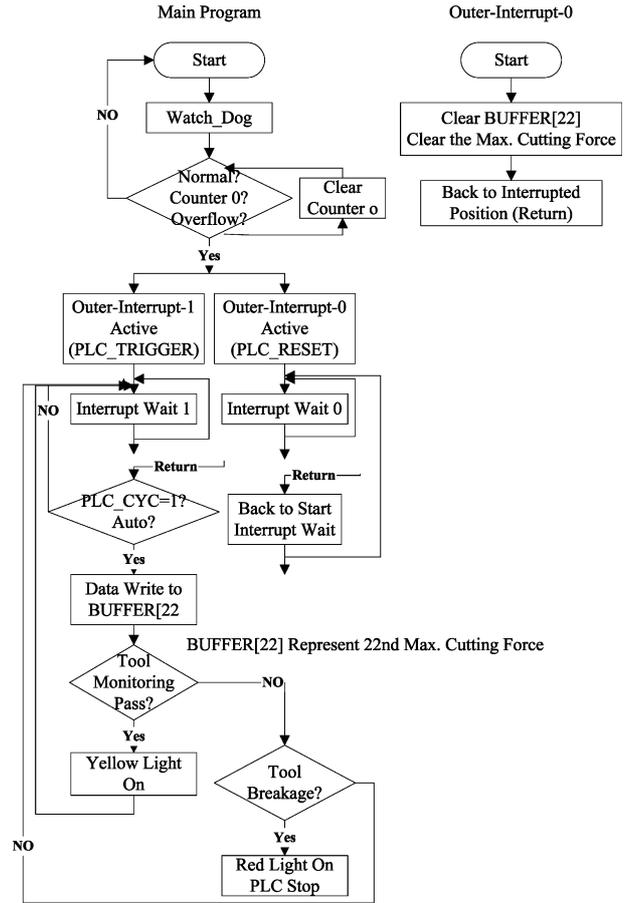
Fig. 3 Tool monitoring program flowchart
