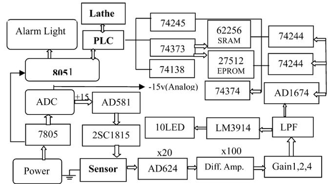
Fig. 2 The hardware circuit of the on-line monitoring single-chip
