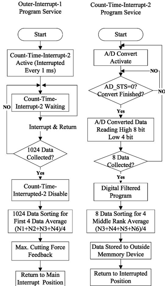
Fig. 4 Detail flowchart of the tool monitoring program
