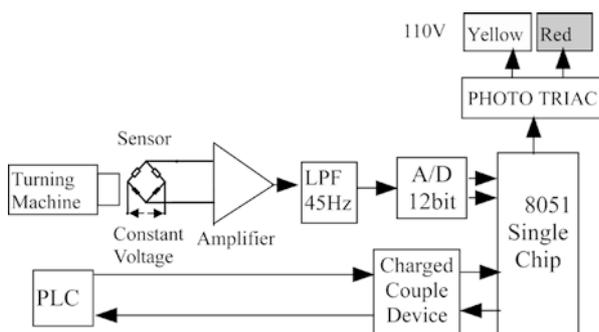
Fig. 1 The diagram of the cutting tool monitoring system structure
